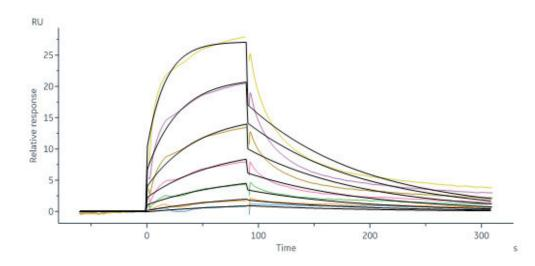
Anti-TREM2 antibody captured on CM5 chip via Anti-human IgG Fc antibodies surface can bind Human TREM2, His Tag (Cat. No. TR2-H52H5) with an affinity constant of 95.9 nM as determined in a SPR assay (Biacore 8K) (Routinely tested).
