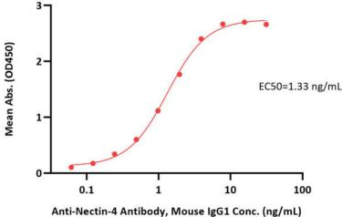
Immobilized Biotinylated Human Nectin-4 (32-153), His,Avitag (Cat. No. NE4-H82Ea) at 1  $\mu$ g/mL (100  $\mu$ L/well) on streptavidin (Cat. No. STN-N5116) precoated (0.5  $\mu$ g/well) plate can bind Anti-Nectin-4 Antibody, Mouse IgG1 with a linear range of 1-4 ng/mL (QC tested).
