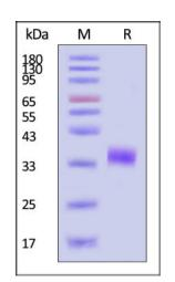
Biotinylated Human CD32b/c, Avitag, His Tag on SDS-PAGE under reducing (R) condition. The gel was stained with Coomassie Blue. The purity of the protein is greater than 95% (With <u>Star Ribbon Pre-stained Protein Marker</u>).
