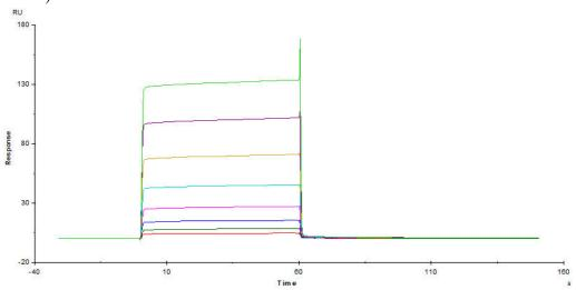
Immobilized Biotinylated Human CD32b/c, Avitag,His Tag (Cat. No. CDB-H82E0) on SA Chip, can bind Rituximab with an affinity constant of 4.22  $\mu$ M as determined in a SPR assay (Biacore T200) (Routinely tested).
